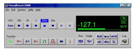
Figure 1-2. NI-DMM Soft Front Panel
